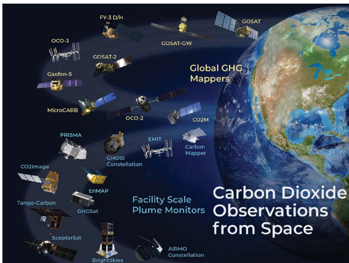
Figure 1: Satellite instruments for observation of methane. Area flux mappers are designed to quantify total methane emissions on regional to global scales. Point source imagers are designed to quantify emissions from individual point sources by imaging the atmospheric plumes
