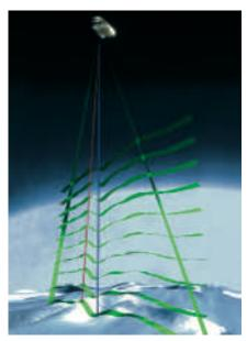
Over topographic surfaces, the first radar echo comes from the nearest point to the satellite. CryoSat can measure the angle from which this echo originates, so that the source point can be located on the ground. This, in turn, allows the height of that point to be determined.
