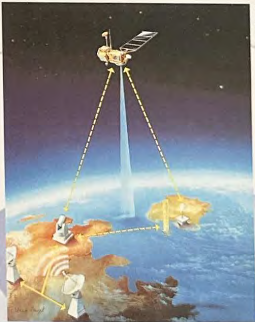
Altimetry satellites, tide-gauge networks, and land and satellite-based geodetic location systems are vital for accurate, long-term continuous monitoring of sea level.
