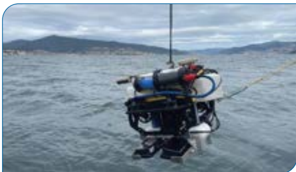
Fig. 5 ROV with instrumentation customized to collect UHI
