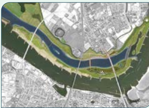
Fig. 2.3 Room for the River Nijmegen: the most complex project within the Room for the River programme. In addition to water management measures such as the creation of a bypass channel with inlets, dyke lengthening, and nature development, this unique project involved the construction of three new bridges. [Attribution: H+N+S Landscape Architects]
