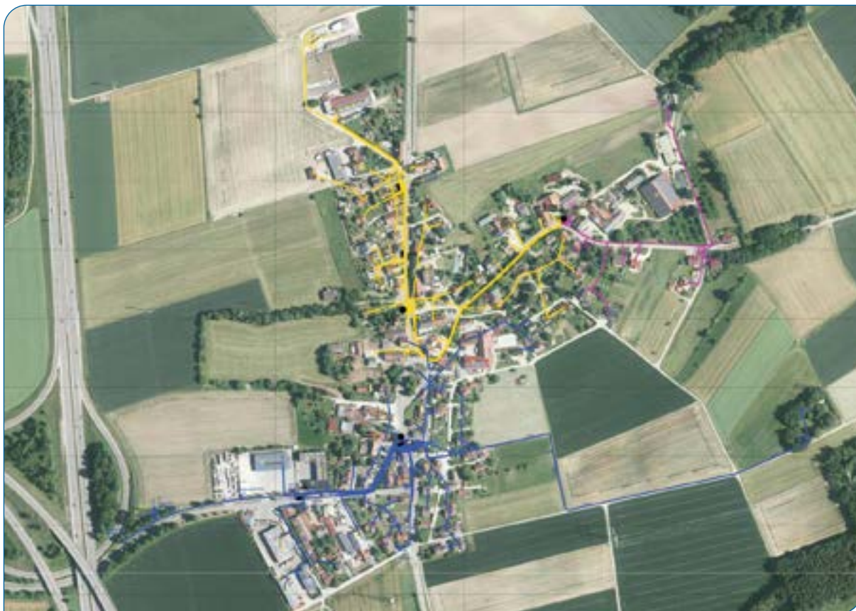
Fig. 1 A power distribution grid at local level: the case of Hittistetten in the city of Senden (Attribution: SWU Netze)
