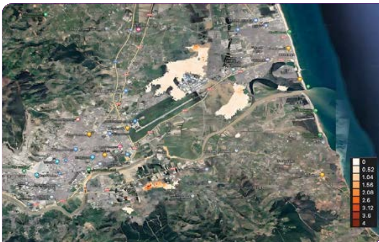
Fig. 5 Water depth computed on the flooded areas. Different colors identify different water depths in meters. Tetouan, Morocco. [Attribution: LIST, CIMA Foundation]
