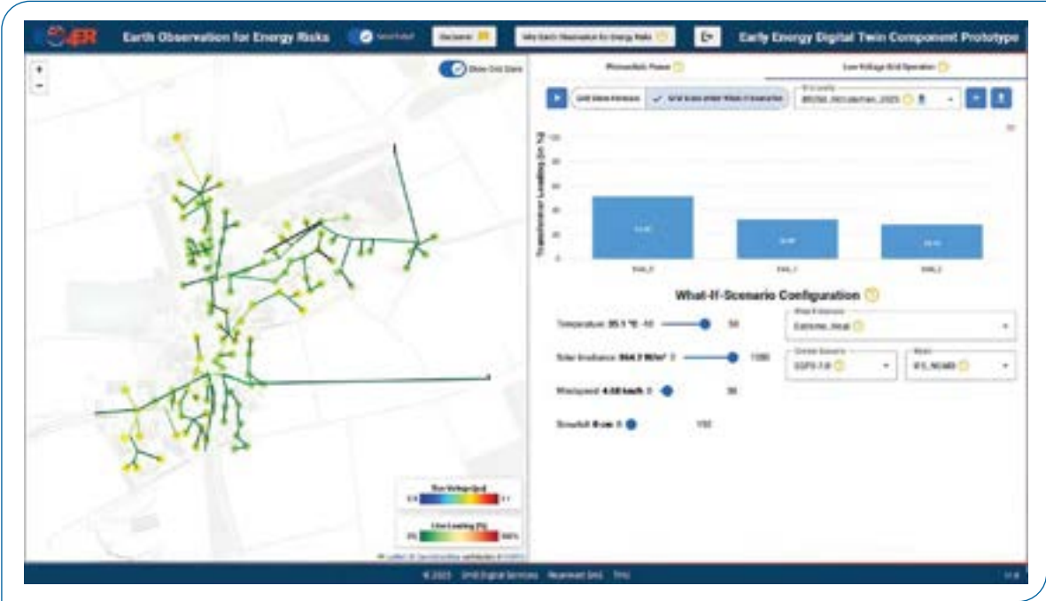
Fig. 3 E04ER's user interface: assessing the state of the grid under climate scenarios
